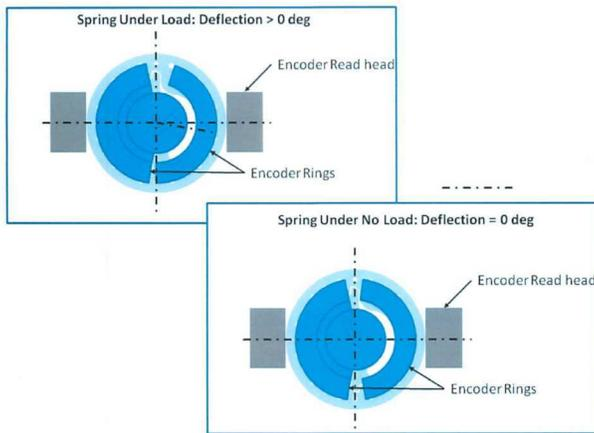
Diagram of deflected (top) versus a non-deflected (bottom) Split-Ring Torque Sensor
