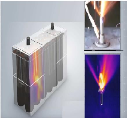
Battery is being tested by inducing the Internal Short Circuit method to one of the cells while introducing heat.
