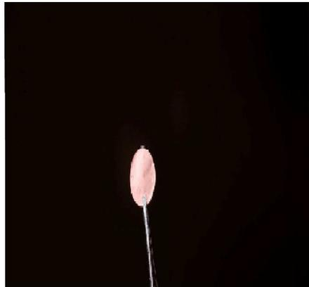
Dime-sized coin made of aluminum and copper is used to induced shot circuits in lithium-ion batteries.
