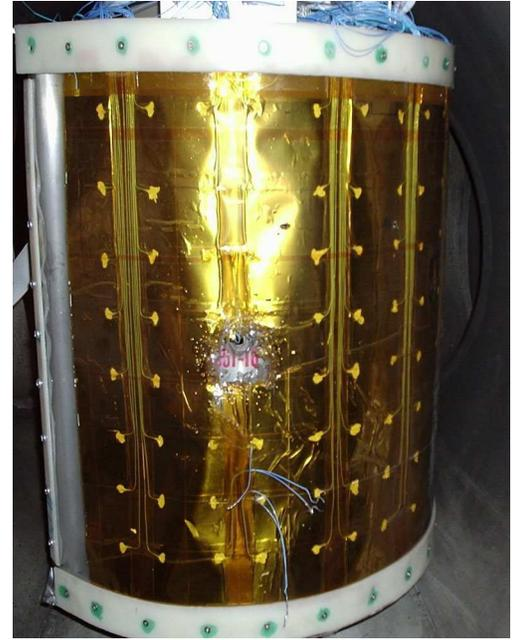
Prototype of the impact detection system after an impact evaluation test.
