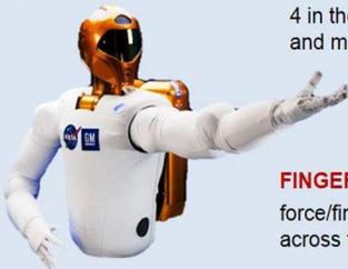
**VISION:** Infrared cameras for depth perception and 4 visible light cameras to provide stereo vision as auxiliary cameras
