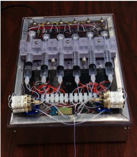
Prototype of the automated system to process biological samples.
