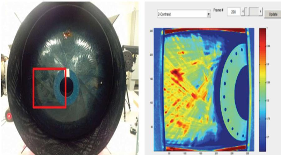
1: Allows for analysis of data in a manner that is similar to pulse/echo ultrasonic testing, making it familiar to technicians
