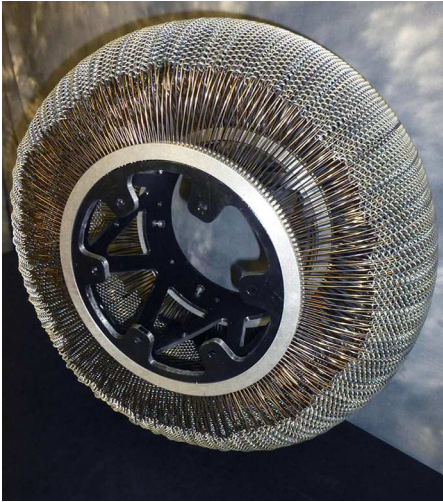
The use of shape memory alloy in radial stiffeners provides even more load carrying potential
