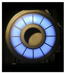
With its flat carbon ion electrodes, Glenn's AIE exhibited superior performance with a thrust-loss correction factor of 0.997, the highest ever demonstrated for an ion thruster
