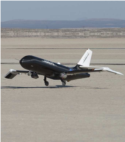
The Spanwise Adaptive Wing provides an all-electric, lightweight, efficient means of deflecting a wing portion to meet flight conditions optimally
