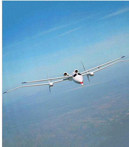
The SAW offers a reusable and reliable alternative to hydraulic systems for actuating wing articulation in subsonic, supersonic, and unmanned aircraft
