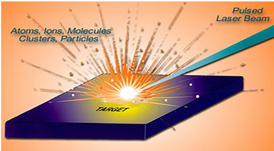
Exposing a surface to a laser beam ablates particles that can be analyzed spectroscopically. Image Credit: NASA
