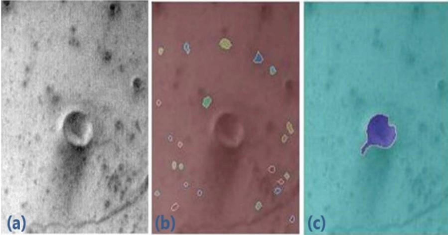
Feature extraction from data collected during the Mars Global Surveyor mission. The original image (a), the close contour features (b) and the elliptic shape features (c) are shown.
