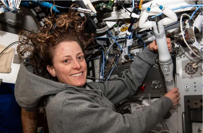
NASA astronaut Loral O'Hara displays spaceMIRA on the space station. The device, a version of the terrestrial surgical system adapted for space, tested techniques for performing robotic surgery in microgravity in February 2024. Credit: NASA
