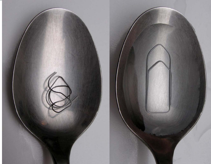
After it deforms, a part made of the alloy nitinol will return to its original shape under a set temperature. This twisted paperclip made of nitinol wire demonstrates how warm water activates the metal memory. Credit: Petermaerki CC BY-SA 3.0
