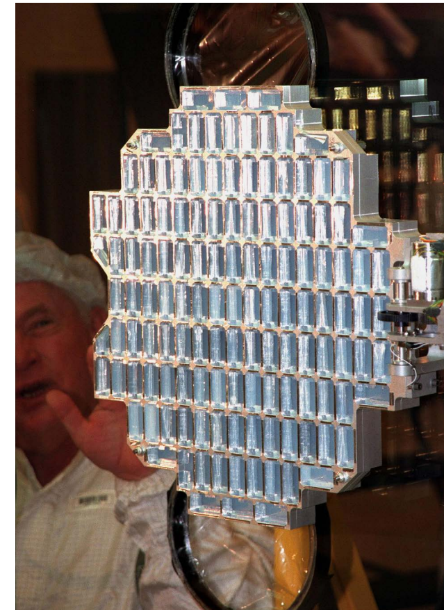
The Jet Propulsion Laboratory perfected aerogel for the Stardust mission. Under Stardust, bricks of aerogel covered panels on a spacecraft that flew behind a comet, with the microporous material "soft catching" any particles that might strike it and preserving them for return to Earth. Credit: NASA
