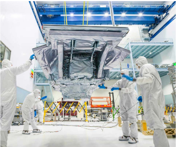
Large parts of the Nancy Grace Roman Space Telescope's Wide Field Instrument are insulated with Integrated Multilayer Insulation. The observatory, which has a field of view at least 100 times larger than that of the Hubble Space Telescope, is expected to launch in 2027. Credit: NASA
