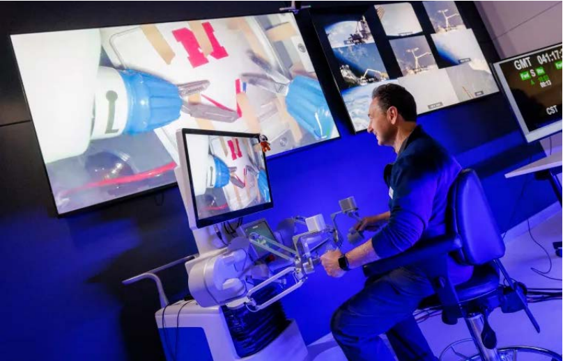
Michael Jobst, a colorectal surgery specialist, makes the first surgical robotic cuts in space from Virtual Incision's offices in Lincoln, Nebraska. For the demonstration on February 13, 2024, surgeons cut rubber bands to mimic surgery inside a payload box on the International Space Station. Credit: Virtual Incision Corp.
