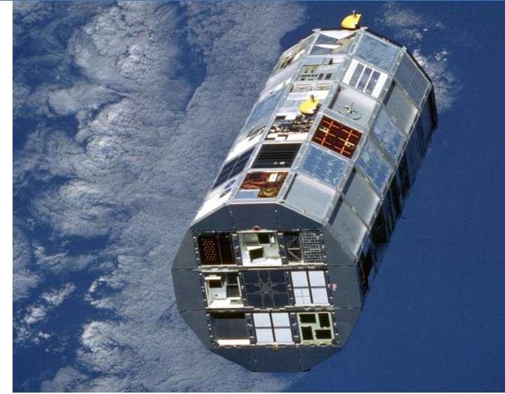
The Long Duration Exposure Facility tested the performance of spacecraft materials, components, and systems in low Earth orbit, exposing them to the environment of micrometeoroids and space debris for an extended period of time. Credit: NASA
