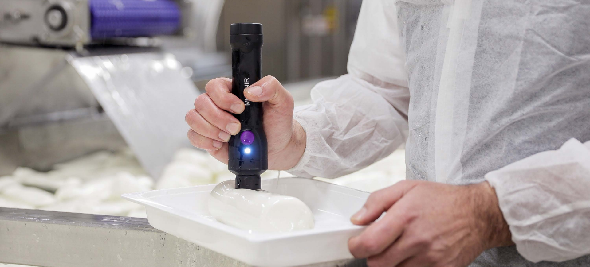
The same filter technology that enables NASA to identify what planets are made of lies at the heart of VIAVI Solutions' Earth-based handheld spectrometers, one of which is pictured here analyzing ingredients in a food production setting. Credit: VIAVI Solutions Inc.
