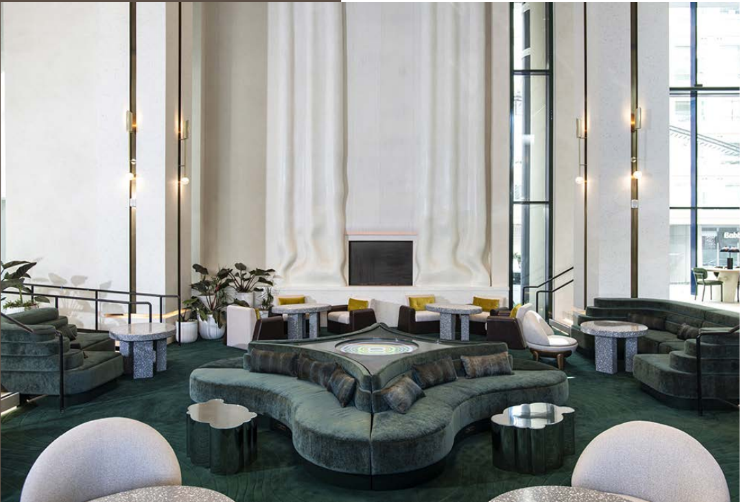
Branch 3D prints lattice structures which can be filled or left hollow to create unique building components, like these drapery-inspired wall panels for the W Hotel in Hollywood. Credit: Branch Technology Inc.
