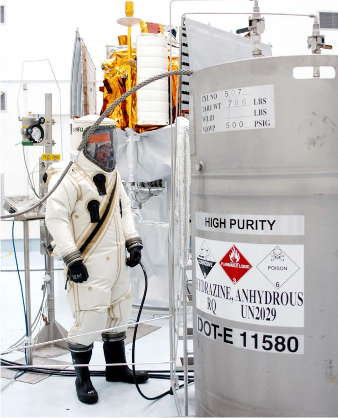
Long-standing satellite propellants like hydrazine are so toxic to humans that workers handling them require a protective suit like this one worn by crew preparing the Mercury Surface, Space Environment, Geochemistry, and Ranging spacecraft. Credit: NASA
