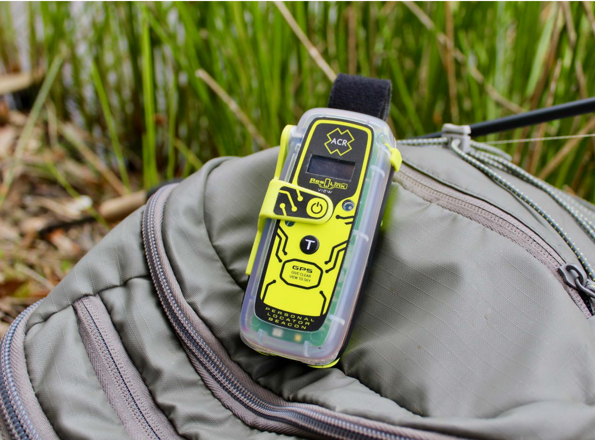
Turning on a ResQLink View PLB from ACR Electronics will automatically "ping" orbiting satellites that send location information to the nearest search and rescue station. Whether on land or water, the appropriate resources will be dispatched to help anyone in distress anywhere in the world. Credit: ACR Electronics Inc.
