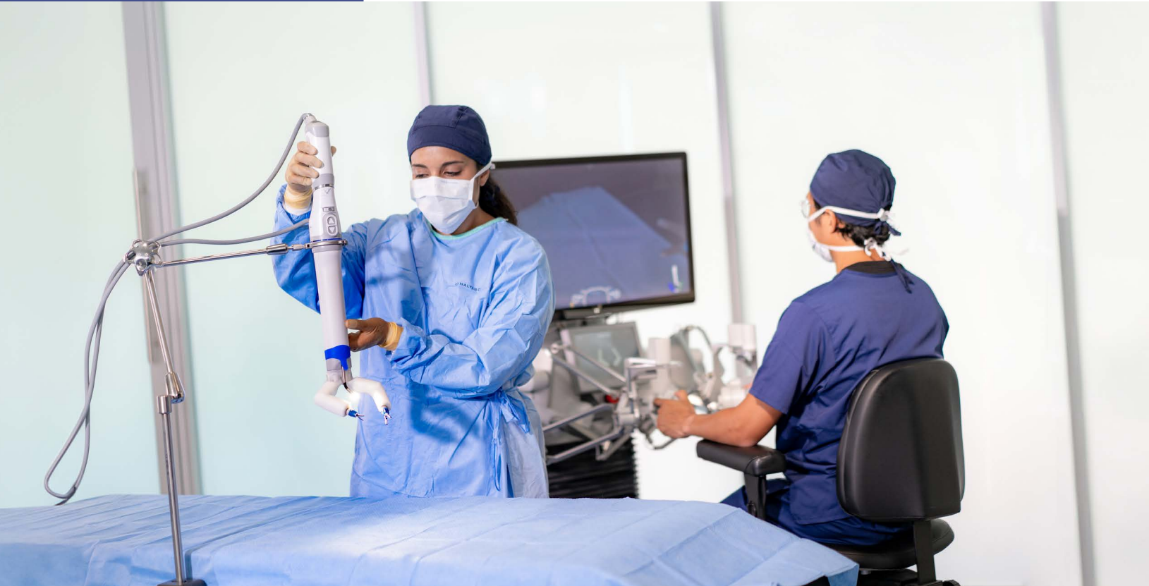
Virtual Incision's MIRA Surgical System enables minimally invasive surgeries and can easily be transferred between operating rooms in a hospital or other surgery site. A surgeon controls the device from a console that's a few feet away or, potentially, much farther. Credit: Virtual Incision Corp.
