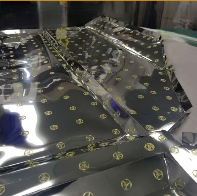
The secret to Integrated Multilayer Insulation is that it replaces the netting that has traditionally separated reflective layers in multilayer insulation with a series of fixed plastic spacers designed to hold everything in place while allowing as little heat conduction as possible. Credit: Quest Thermal Group LLC
