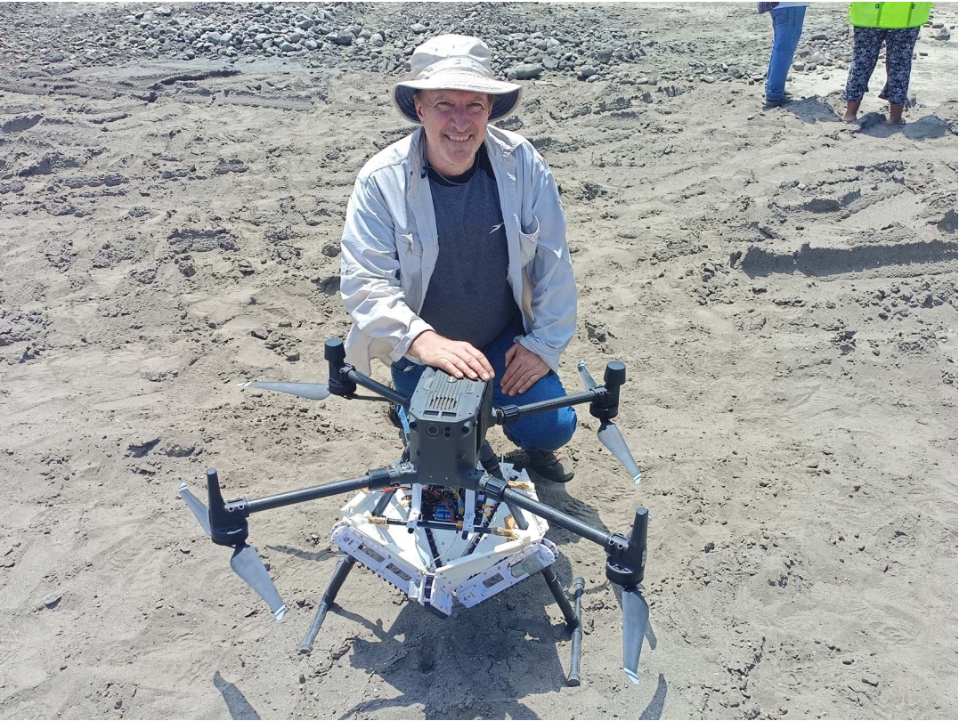
Fletcher poses with the Flying Forests drone he outfitted with a rapid-fire launcher to carpet 25 acres of deforested Peruvian jungle with balls containing the seeds of a hearty legume species. Credit: Beta Earth LLC
