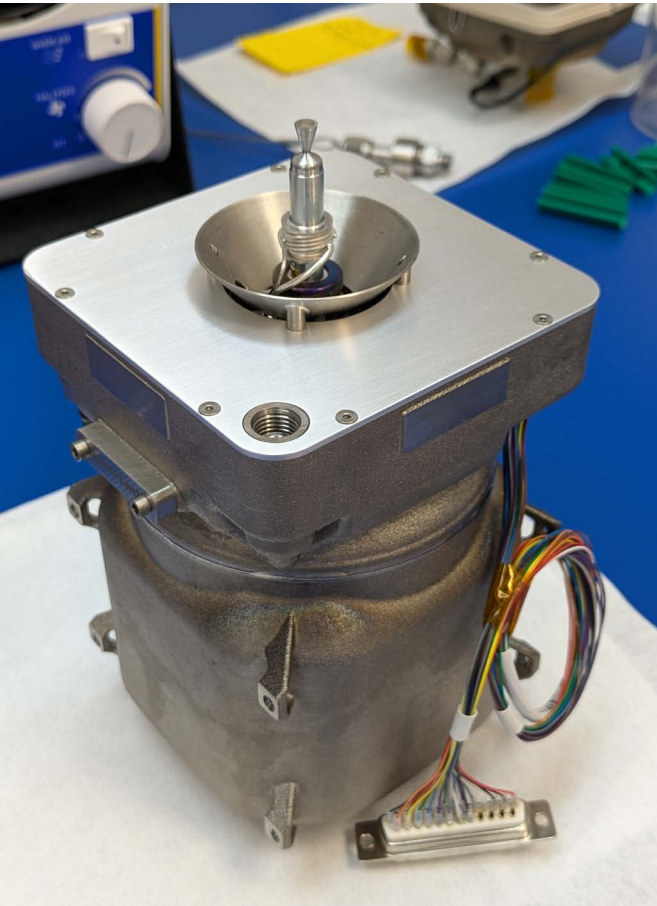
The Sprite propulsion system built by Rubicon Space was developed with NASA to use ASCENT fuel. It's both safer and more efficient than conventional fuel like hydrazine. Credit: Plasma Processes LLC
