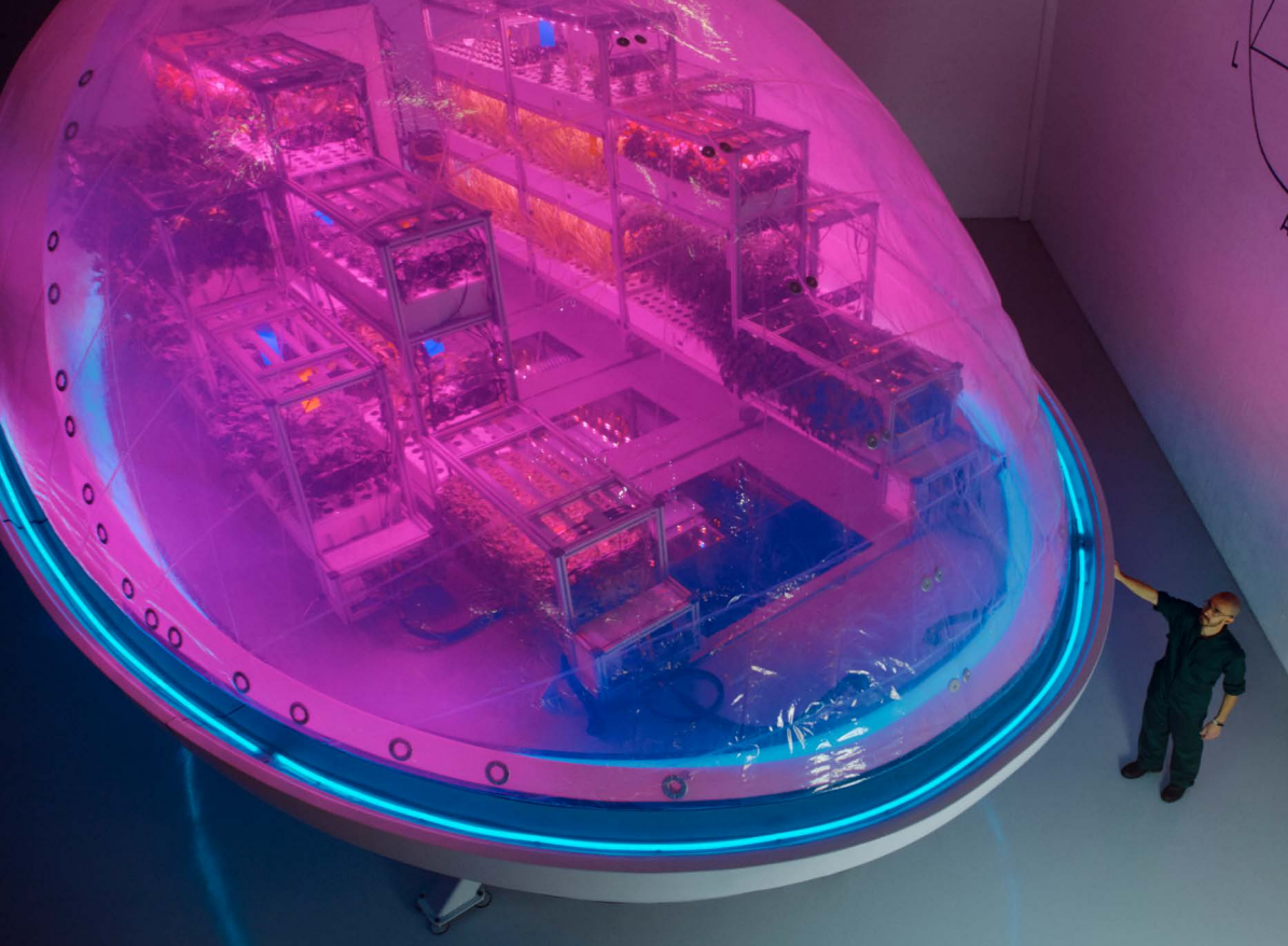
The BioPod, a 17-foot-long, 8-foot-tall precision agriculture device pictured here, was developed by Interstellar Lab to hone the molecular composition of plants, isolating and enhancing particular nutrients or essences. Credit: Interstellar Lab Inc.
